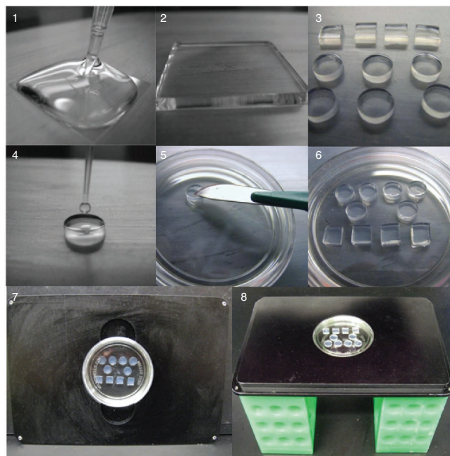
Figure 1 | Slide preparation. (1) Melted agarose is pipetted onto a cover glass (22 mm 2 ). (2) Two cover glasses make an agarose ‘sandwich’ of even thickness. (3) Smaller agarose pads are cut from a larger pad. (4) Bacteria are loaded on top of the pads. (5) After drying, pads are flipped and transferred to an imaging dish. (6) Many pads can be loaded on a single dish. (7) After sealing with Parafilm or grease, the dish is placed into a custom stage insert that holds the dish tightly. (8) When manufactured precisely, the stage insert can be turned upside down without the dish falling out, thereby allowing imaging with an upright microscope.
